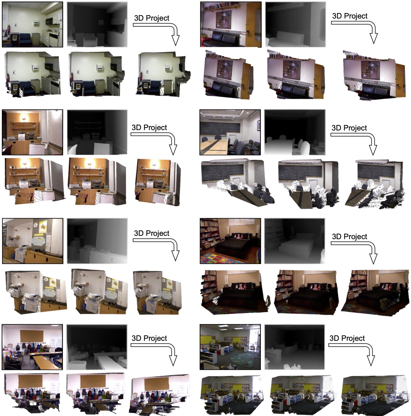
Figure 30. Potential application of single-view scene reconstruction. Given an RGB image and predicted depth map, we lift this image into a 3D space. We illustrate three views of this scene. Best viewed in color.
